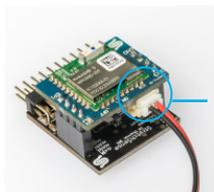
Plug in battery and turn on the Bluetooth low energy board with the toggle switch.
